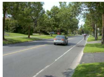
Example dedicated on-street bike lane
